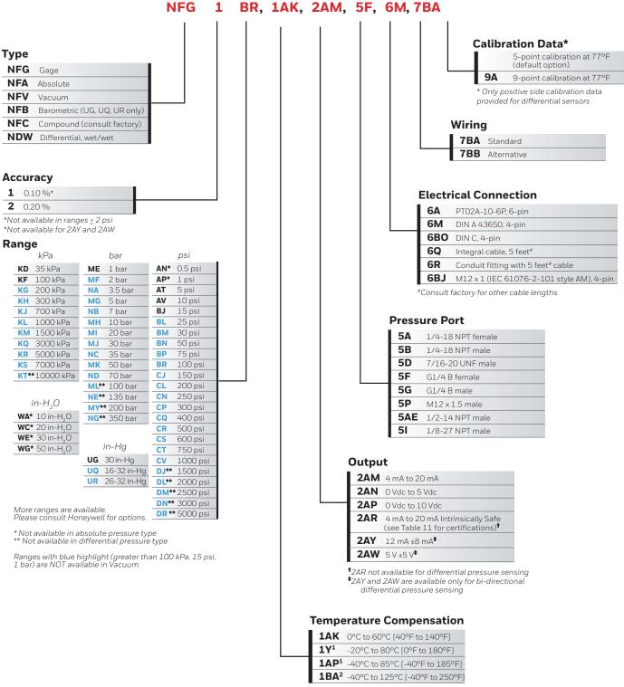
$<sup>^1\,</sup>$  1Y and 1AP not available for pressure ranges below 5 psi [0.35 bar]  $^2\,$  1BA not available for pressure ranges below 50 psi [3.5 bar]
