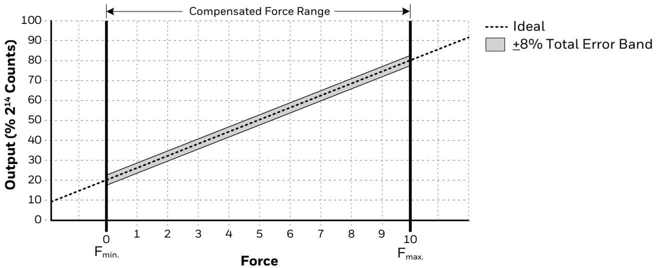
$$\text{Output (\% of } 2^{14} \text{ counts)} = \frac{60\%}{\text{Force}_{\text{range}}} \times (\text{Force}_{\text{applied}}) + 20\%$$
