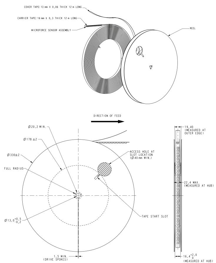
FIGURE 5. TAPE MOUNTING DIMENSIONS (FOR REFERENCE ONLY: MM/[IN], ALL DIMENSIONS COMPLY WITH EIA-481-1.)
