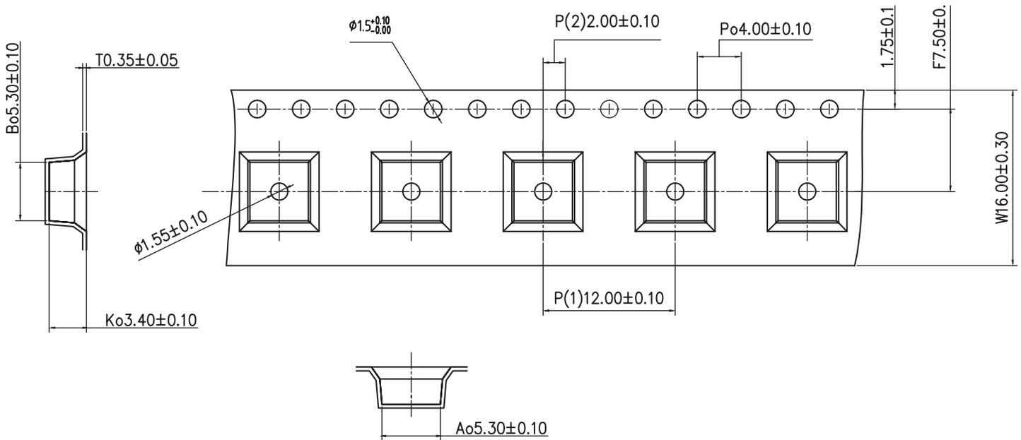
Note: FMA Series products are shipped in tape and reel packaging with a Minimum Order Quantity (MOQ) of 160 pieces. The maximum tape and reel quantity is 960 pieces per reel.
